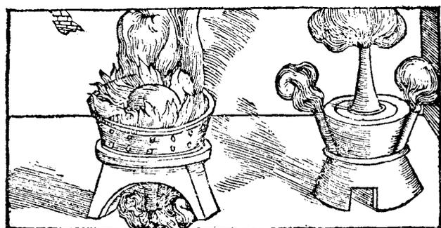
FIGURE 6. Two types of apparatus for sublimation; left, by descent; right, by ascent, the type suitable for the preparation of vermilion from mercury and sulphur. From Vannoccio Biringuccio, *De la pirotechnia*, Venice 1540.
